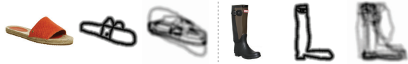
Figure 3. Overfitting examples in the training dataset. Images from left to right are input images, reference sketches, and generated sketches. The network is trained with only 10% of the paired data. Sketch patterns of other shoes can be seen in the generated sketches.
