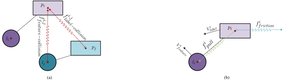
Fig. 4 Basic forces. (a) Repulsive forces between labels and repulsive forces between labels and features, (b) pulling forces between labels and the corresponding features and the friction force
