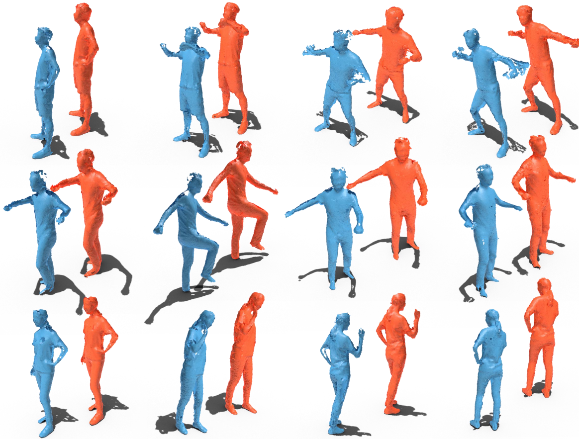
Fig. 7 Selected frames demonstrating the overall reconstruction quality of HDR-Net-Fusion (Rows from top to down correspond to human0/3/8 in Human10, respectively). In each pair of meshes in each row, we show the reconstructed result without HDR-Net in blue and the result with HDR-Net in red. Our algorithm successfully identifies the missing or noisy regions and refines them reasonably.
