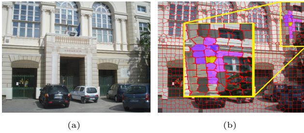
Fig. 5 Illustration of generating new labels for unreliable superpixels. Image (a) shows The original input image I_1 , while image (b) shows the process of searching similar superpixels in R . The dark region in (b) shows the unreliable superpixels, and the yellow one represents the unreliable superpixel to be processed. The blue ones are the most similar superpixels of the yellow one we searched from R .
