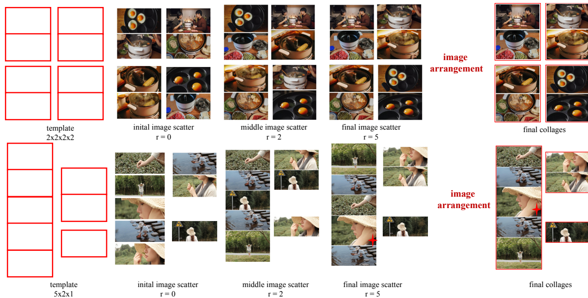
Fig. 5 Pipeline of template-fixed collage generation. The fixed template is sketched out with red boxes, and the uniqueness image is labeled with red star. As the number of iterations ( r ) increases, the collages gradually become clear and tidy information, which leads to a visually easy and pleasant experience.
