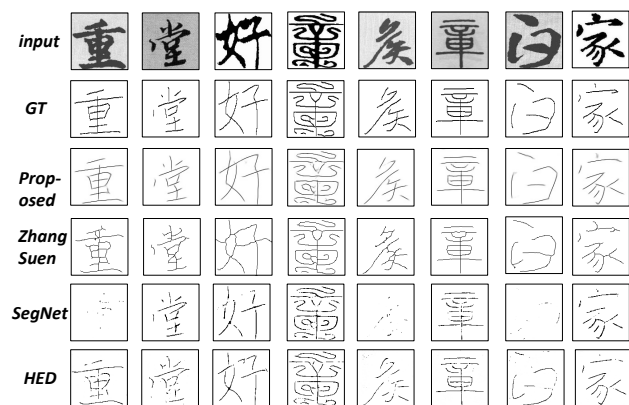
Fig.11. Skeletons extracted for real-world calligraphic characters (input) by the proposed approach (proposed) and the three peer methods with respect to the groundtruth (GT).
