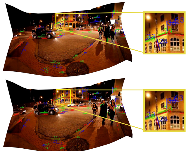
Fig. 4 The lines structure and matching between two successive frames. The corresponding lines are denoted by the same indices.
