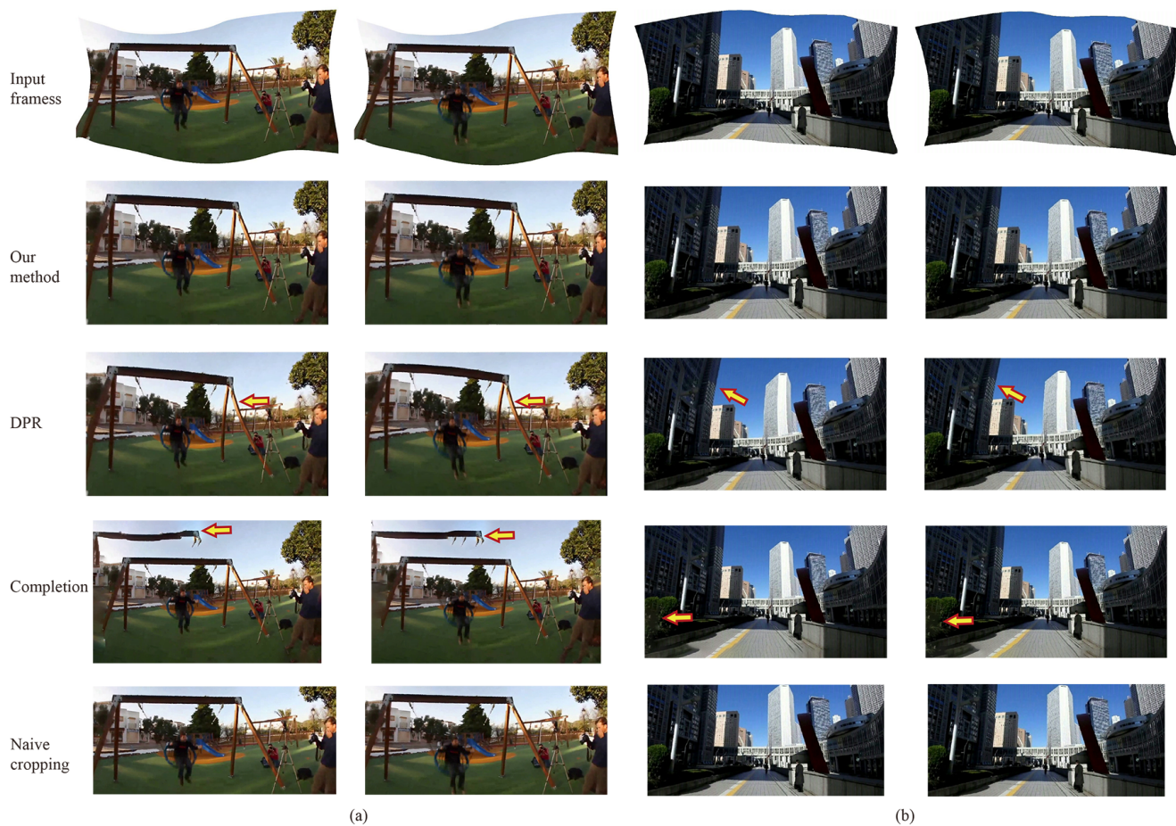
Fig. 6 Comparison of rectangling distortion-corrected fish-eye videos. From top to bottom: input frames of two examples; rectangling results by our approach, DPR [35], video completion method [33] and naive cropping results.
