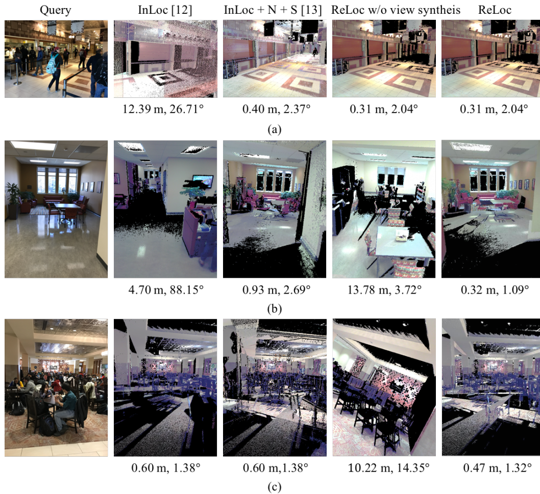
Fig.5. Three Qualitative examples of visual localization on InLoc dataset. The query images of 3 examples are in left column, the right 4 columns show the localization results of InLoc, InLoc+N+S, and proposed method without and with view synthesis, respectively. It is obvious that the proposed method outperforms the others, and in which the view synthesis matters.
