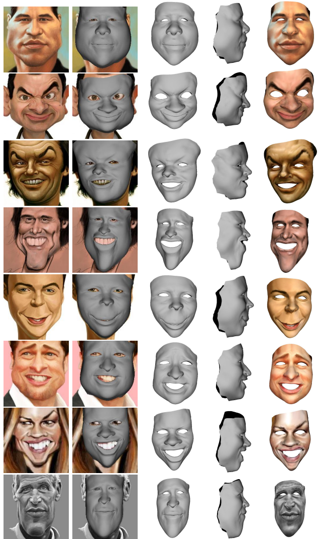
Figure 8. Left to right: input caricature, predicted mesh overlaying on the image, predicted mesh in two different views, predicted mesh with texture.
