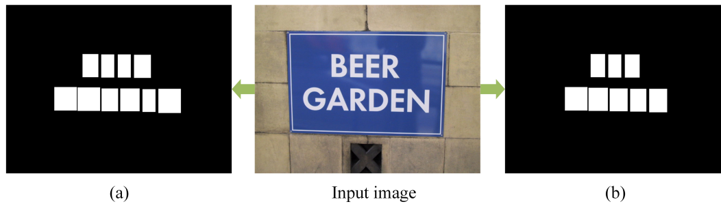
Fig.7. Annotation of (a) character instances and (b) character affinity. For this input image, 4 character boxes and 3 character affinity boxes are generated for “BEER”, and 6 character boxes and 5 character affinity boxes for “GARDEN”.
