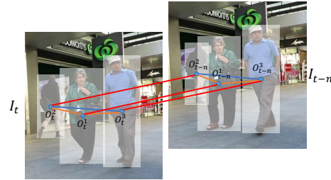
Figure 4. The node association and edge association between two object graphs of I_t and I_{t-n} . The red solid line represents the object node that is successfully matched by the node association strategy; the orange solid line represents the structural similarity information of the object node learned by the edge association strategy.
