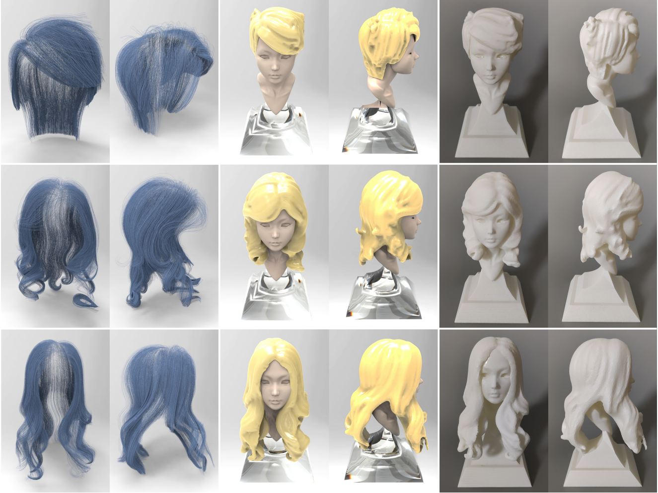
Figure 7: Reconstructed and 3D printed results from strand-level hairstyles. From left to right: input strands in two views, reconstruction results, and 3D printed results.
