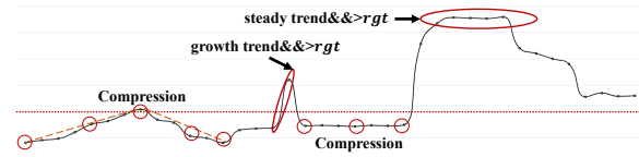
Fig. 5 Features of communication latency over time, which are used to generate temporal latency abstraction using the sliding window algorithm. The red line denotes gt_{region} , and the important growth trend period and steady trend period are circled by ellipses. The other features are compressed (reserve part of the data).
