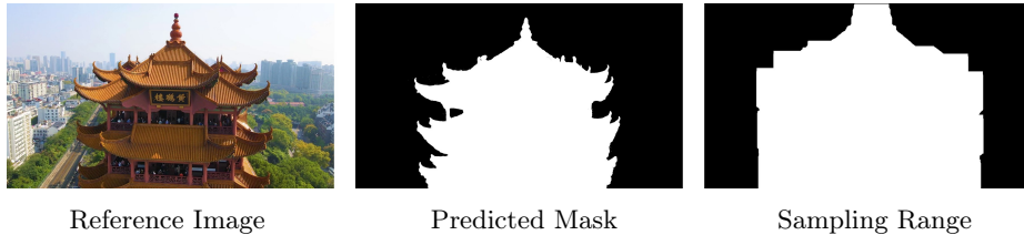
Fig. 2: From left to right: Original image, the foreground mask predicted by the network, final sampling range after image processing. For not generating artifacts in the edge area of the reconstructed object, the sampling range is larger than the predicted mask.
