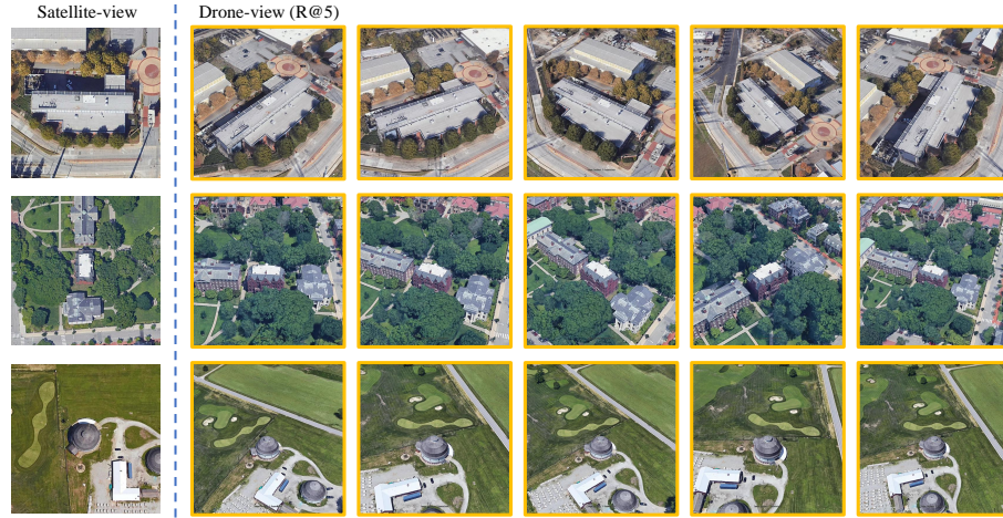
Fig. 7. Visualization of drone-view target localization. Inputting the drone-view images as the query images, we show the top 5 satellite-view images in the ranking of the matching results in the drone→satellite task.
