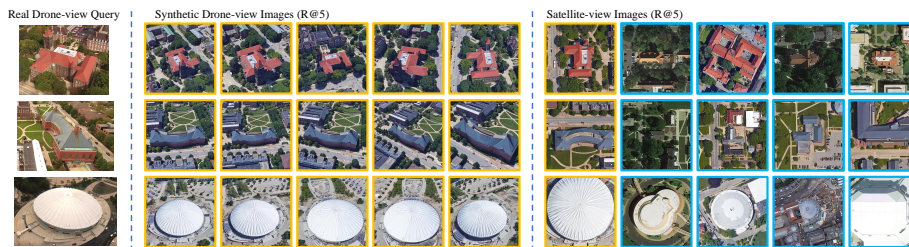
Fig. 9. Qualitative image search results using real drone-view query. In the left column, we show the real drone-view images used for the query. In the middle column, we show the top-5 most similar images in the test set retrieved by our model. In the right column, we show the retrieval results for drone-view target localization.
