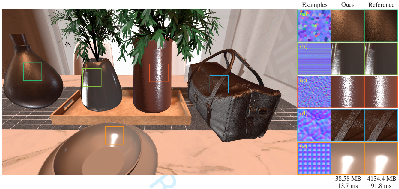
Fig.6. The comparison between our method and the reference method [1] on the Desktop scene with various types of microstructures. The high-frequency effects are almost identical. Our method only consumes 1% of memory overhead and significantly improves the rendering speed compared to the reference.
