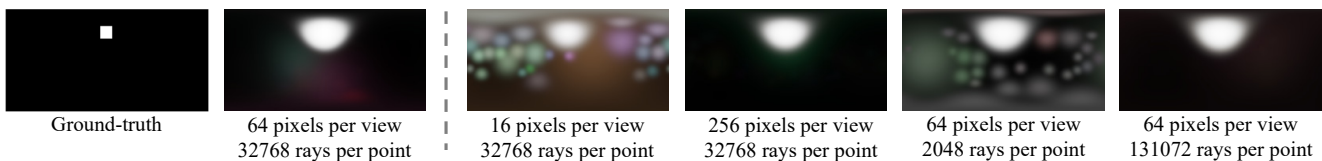
Figure 5. Estimating environment lighting by different sampling strategies. All the results are estimated in DOG. The result of our proposed method is shown on the second from left, which samples 64 pixels per view and traces 32768 rays at each surface point corresponding to the pixel. Results estimated by other sampling strategies are shown on the right side of the dashed line.
