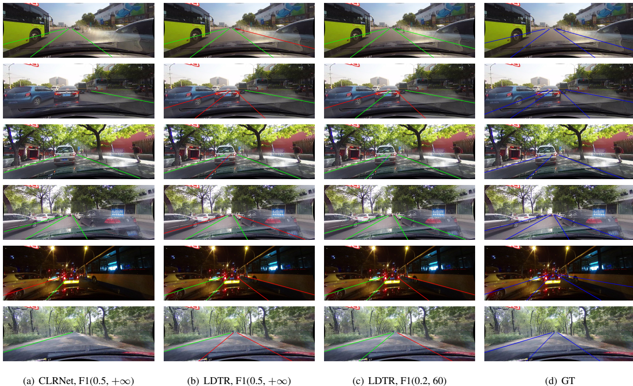
Fig. 14 Prediction ability comparison between CLRNet and LDTR for “Congested Scenarios” in CULane. The green and red lines represent the true positive (TP) and false positive (FP) of the model’s prediction results under a specific evaluation indicator, respectively, while the ground truth (GT) is represented by blue lines.
