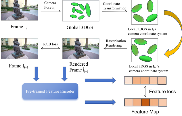
Figure 2. Overview of the Relative Camera Pose Optimization Module for Ordered Frame Sequences. We use the global 3DGS of the known frame to obtain the pose and image of the next frame through coordinate transformation and rendering, and introduce feature loss and RGB loss to optimize the relative camera pose, thereby achieving noise-robust pose estimation.
