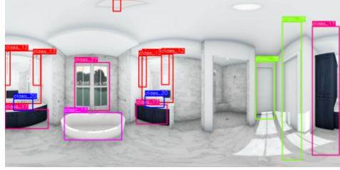
Figure 3. Effect of annotating in spherical space with planar boxes and then converting to an ERP image.
