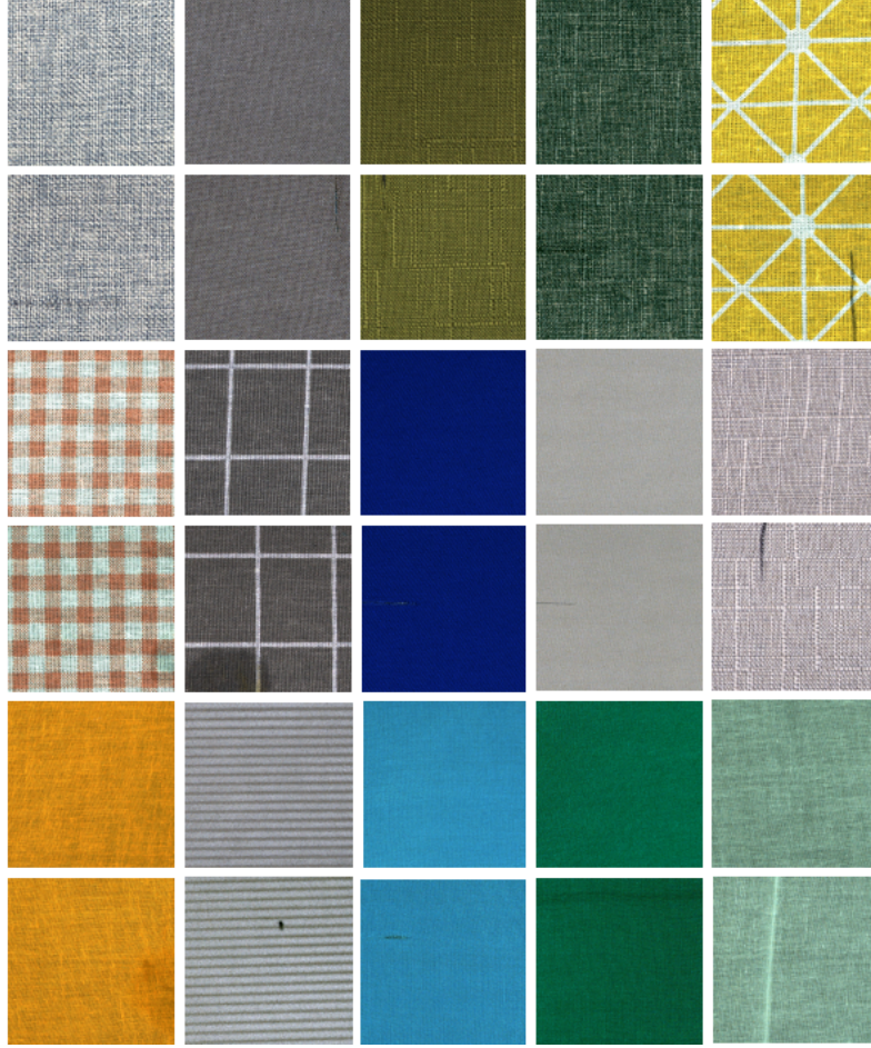
Figure 3: Example images of all fifteen different colors and textures of cloth from the Texture-AD dataset. For each category, the first row displays anomaly-free examples. The second row shows examples of the anomaly.
