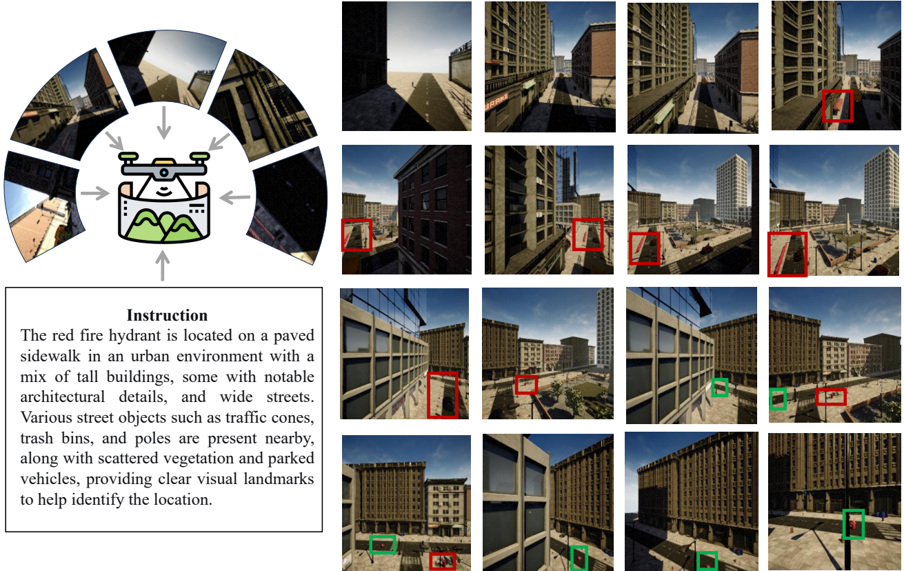
Figure 1. Task definition for UAV navigation. This set of images shows the target recognition process for a UAV in a simulation environment. The red boxes represent negative samples, which are distracting objects whose color or shape might cause confusion (such as traffic cones and trash cans). The green boxes represent positive samples, which are fire hydrants that need to be located.
