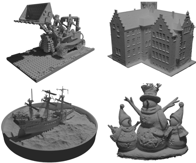
Fig. 1. We present PGT-NeuS, a neural reconstruction method that performs exceptionally well in multi-views reconstruction of exquisite geometric details. Leveraging the proposed progressive-growing tri-plane representation, our method can capture delicate surface details across different objects, achieving high-precision reconstruction. We highly recommend readers to zoom in and observe the details.
